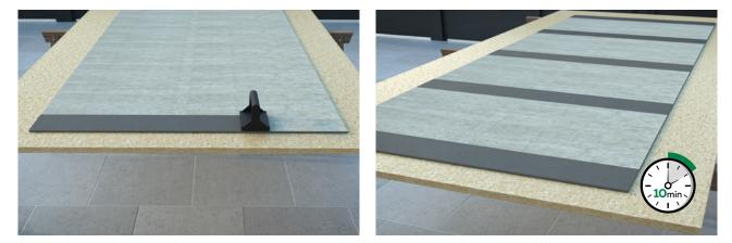
2. Apply Innotec<sup>®</sup> Imprisol Project Primer on the cleaned areas of the backside of the Hardie<sup>®</sup> Panel - Waiting time 10 minutes.
