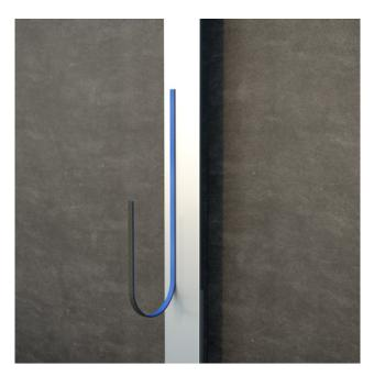
Attach the Innotec<sup>®</sup> Fixation Tape Project 2100 to the sub-frames. The tape should be aligned towards the joint, leaving sufficient space for the Innotec<sup>®</sup> Adheseal Project adhesive triangle (8 mm), see 9 for the correct alignment.
